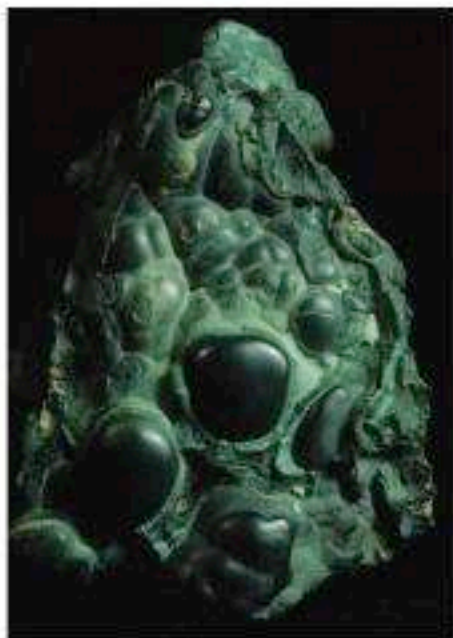
Figure 22.5 Malachite is a copper ore. You can think of it as behaving like a mixture of copper(II) carbonate and copper(II) hydroxide.
