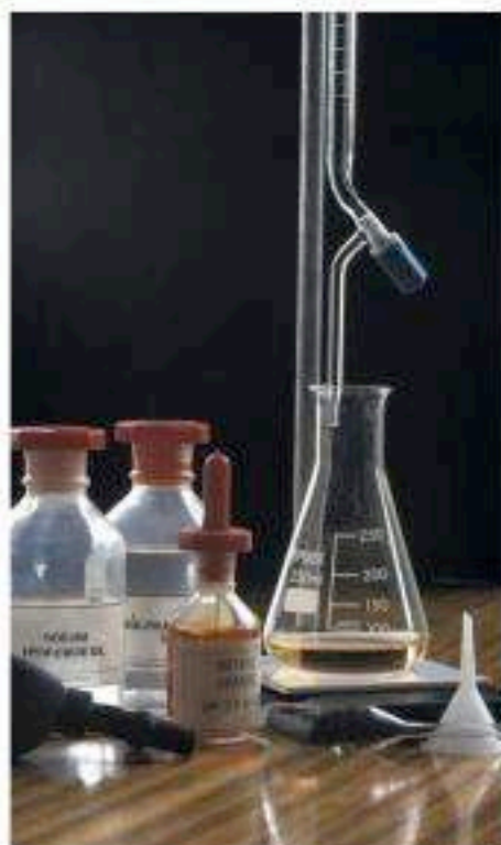
Figure 10.9 Apparatus for carrying out a titration.
