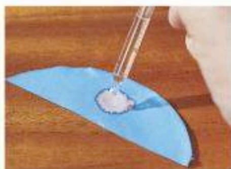
Figure 11.12 Testing for water with cobalt chloride paper.
