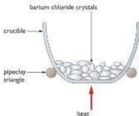
Figure 22.12 Heating barium chloride crystals in a crucible.
