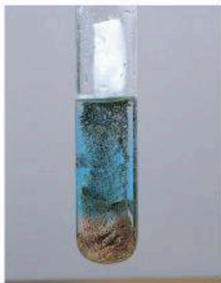
Figure 8.8 Zinc displaces copper from copper(II) sulfate solution.
