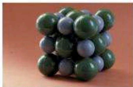
Figure 4.11 A model of a small part of a sodium chloride crystal.
