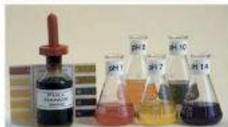
Figure 9.4 Using universal indicator solution to measure the pH of various solutions.
