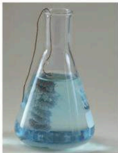
Figure 8.10 Displacing silver from silver nitrate solution.
