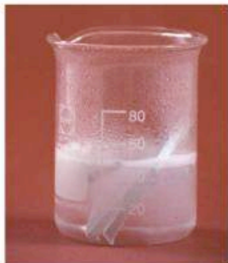
Figure 10.5 Dilute sulfuric acid with excess magnesium.
