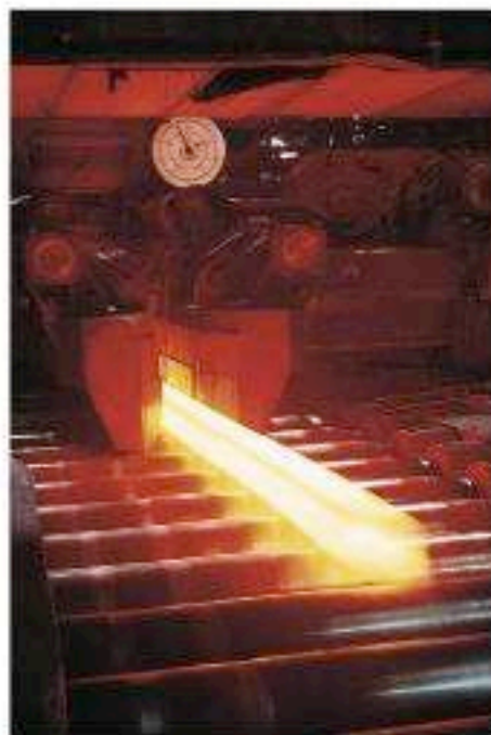
Figure 4.8 Steel being rolled into strips.
