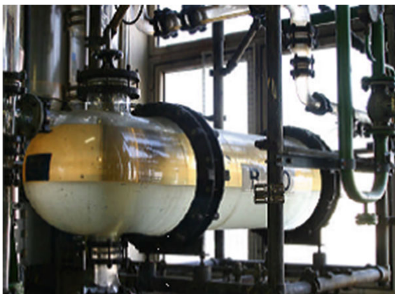
Fig. 20.15 BASIL process with a much smaller jet reactor. Image copyright from BASF—The Chemical Company
