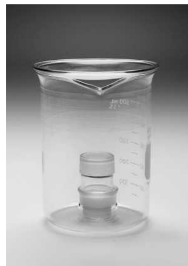
Figure 2-9 Arrangement for the drying of samples.
