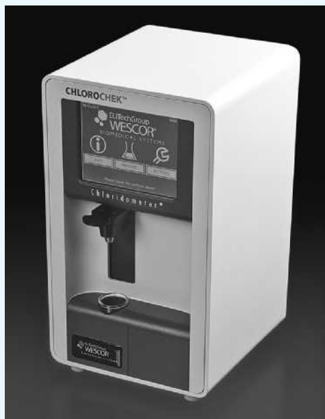
Figure 22F-2 A commercial digital chloridometer. This coulometric titrator is used to determine chloride ion in clinical samples and in food and environmental samples. The end point is detected by a pair of electrodes measuring solution conductance (Courtesy of Wescor, GMBH, Berlin).
