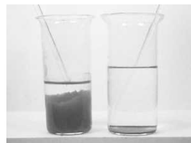
Figure 12-5 Aluminum hydroxide formed by the direct addition of ammonia (left) and the homogeneous production of hydroxide (right).
