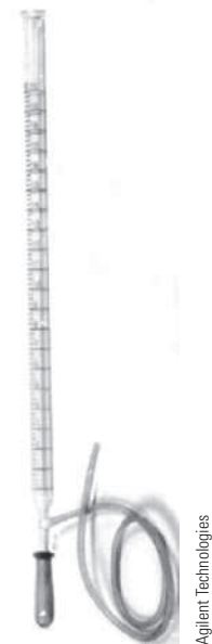
Figure 32-2 A soap-bubble flow meter.
