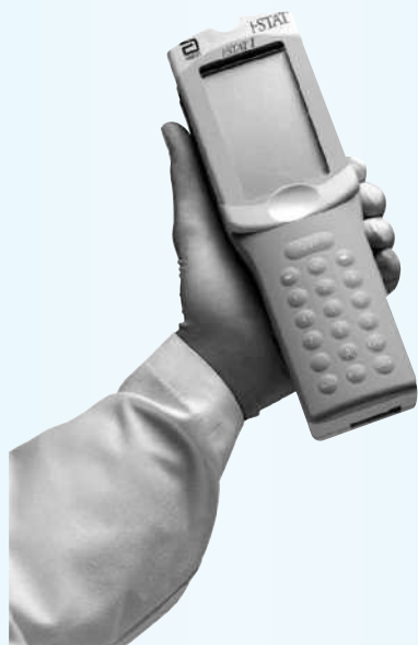
Figure 21F-4 Photo of iSTAT 1 portable clinical analyzer. (Courtesy of Abbott Point of Care, Inc., Princeton, NJ.)
