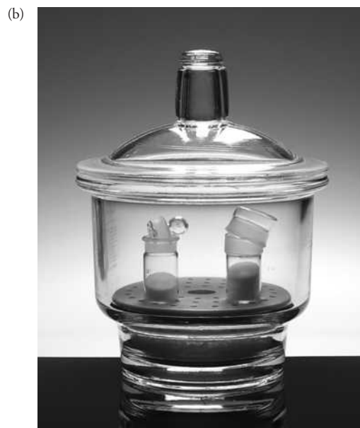
Figure 2-8 (a) Components of a typical desiccator. The base contains a chemical drying agent, which is usually covered with a wire screen and a porcelain plate with holes to accommodate weighing bottles or crucibles. (b) Photo of desiccator containing weighing bottles with dry solids.
