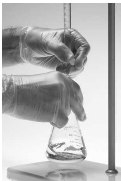
Figure 2-23 Recommended method for manipulating a buret stopcock.
