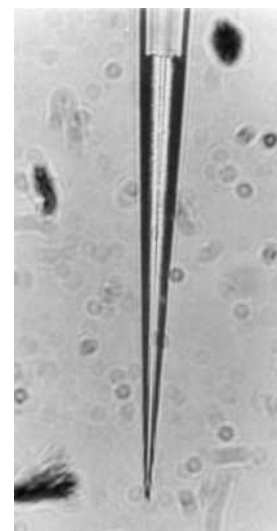
Figure 21-14 Photograph of a potassium liquid ion exchanger microelectrode with 125 \mu\text{m} of ion exchanger inside the tip. The magnification of the original photo was 400 \times . (Reprinted with permission from Anal. Chem. , March 1971, 43(3), 89A-93A. Copyright 1971 American Chemical Society.)
