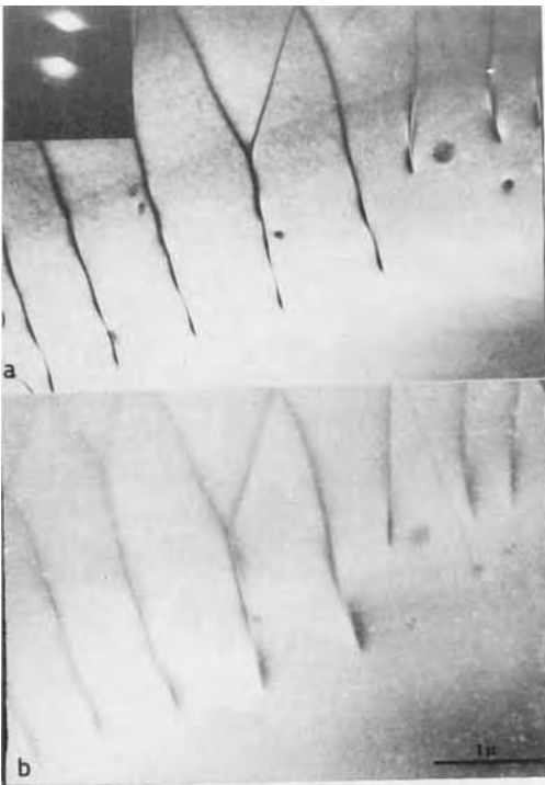
Figure 61. Dislocations in \text{SnS}_2 exhibiting oscillating contrast on approaching the surface: (a) bright field image; (b) dark field image. (Courtesy of P. Delavignette.)
