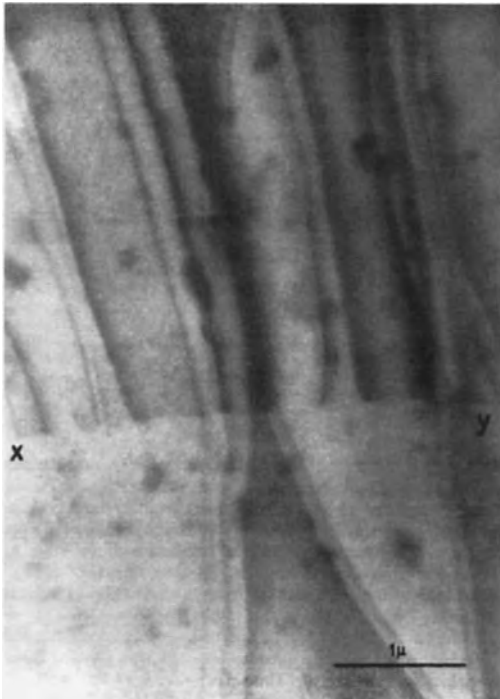
Figure 11. Triple ribbon in the (0001) plane of graphite passing under a surface step XY, hereby changing its width (TEM) (Amelinckx et al. [42]).
