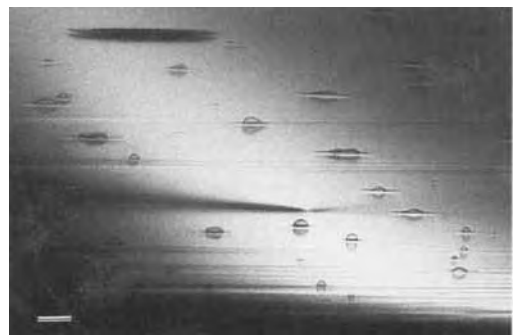
Figure 7. REM image of small transparent foreign particles on an Si (1 1 1) surface showing the direct image and mirror image and the bright line between them in each case (plus a dislocation strain field). Scale bar: approx. 50 nm. (Courtesy of T. Hsu.)
