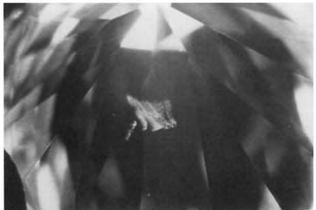
Figure 18. Typical example of a 'cloud' in a diamond. Clouds consist of numerous, very small, pinpoint inclusions.
