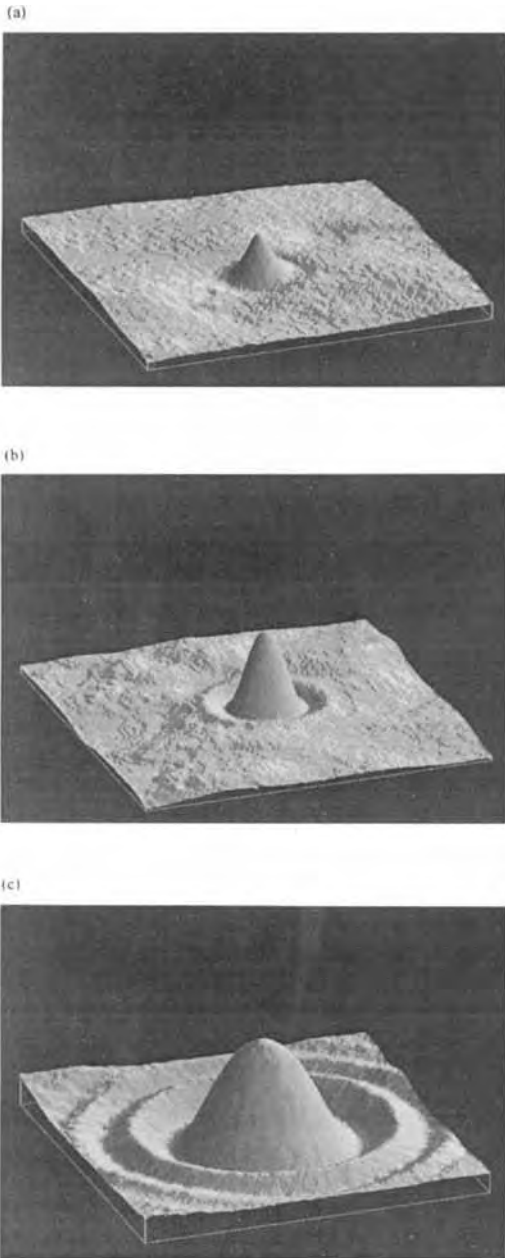
Figure 17. Shock propagation on a plate ( 45 \times 45 cm). The three-dimensional images show a sequence of deformation hillocks by using interferometry. The hillock heights are (a) 0.7 \mu\text{m} , (b) 1.1 \mu\text{m} , and (c) 1.2 \mu\text{m} . (Courtesy of Steinbichler Optotechnik GmbH, Neubuern, FRG.)
