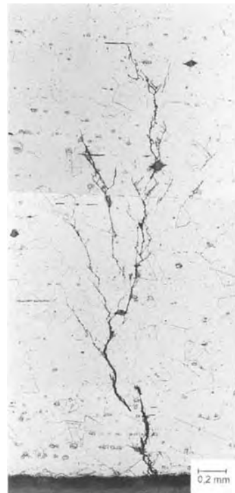
Figure 25. TRSCC caused by local contamination with chloride-containing impurities in a tube of the austenitic stainless steel 1.4550.
