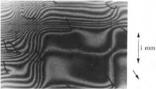
Figure 9. Synchrotron radiation topograph of silicon on insulator (Simox) sample, consisting of (100) silicon substrate, 550 \mu\text{m} thick, with 0.4 \mu\text{m} layer of \text{SiO}_2 and 15 \mu\text{m} of Si epitaxially grown on top. (040) reflection, \lambda = 0.3 \text{ \AA} , exposure time 1000 s on HR film. Dislocations in the substrate, misfit dislocations, and moiré fringes are visible. (Courtesy of Eetu Prieur, ESRF.)
