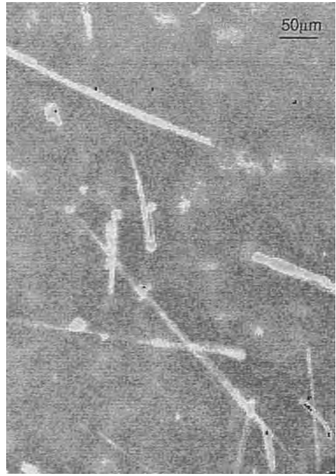
Figure 11. Zinc precipitates in a magnesium matrix obtained with an electronic camera in XPM (see Fig. 10). (Photo: Courtesy of H. Elhila.)
