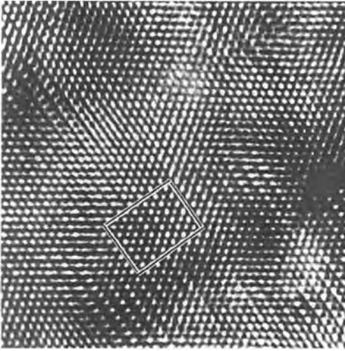
Figure 4. TEM micrographs of \langle 110 \rangle oriented \text{Cu}_3\text{Au} after 400-keV electron irradiation at total doses of 2.3 \times 10^{27} \text{e m}^{-2} (left) and 3.7 \times 10^{27} \text{e m}^{-2} (right) [8].
