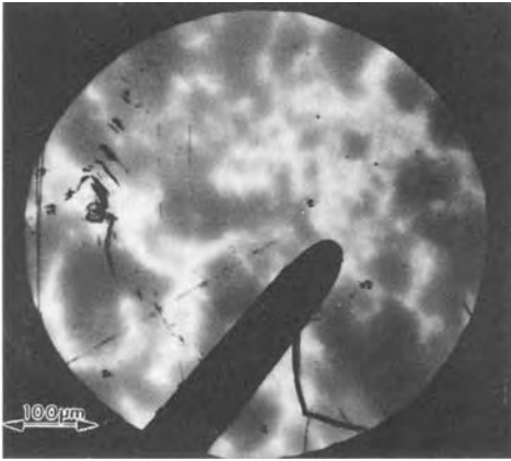
Figure 17. EBIC image of doping variations in GaAs wafer. Recorded in Cambridge S250 SEM at 15 keV.
