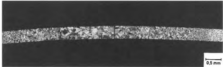
Figure 38. TIG weld on a longitudinal welded tube of Zircaloy 4.
