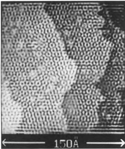
Figure 8. Scanning tunneling microscope image of the surface structure of an Al–Cu–Co decagonal crystal. Ten-fold and quasiperiodic arrangements on several atomic layers are obvious. (Courtesy of Drs A. R. Kortan and H. S. Chen and reproduced from Phys. Rev. Lett. [25].)
