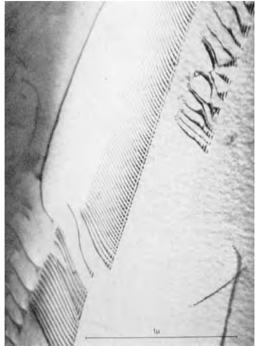
Figure 89. Ribbons dissociated in Shockley partials observed in a Cu-Ga alloy. (Courtesy of A. Art.)
