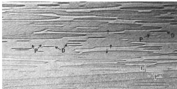
Figure 1. REM image of one-atom high surface steps on a Pt (111) surface. Arrows indicate the step-down direction. Circular features, foreshortened to thin ellipses, are atom-high projections, P, or depressions, D. Note the intensity changes across the steps. (Courtesy of T. Hsu.)
