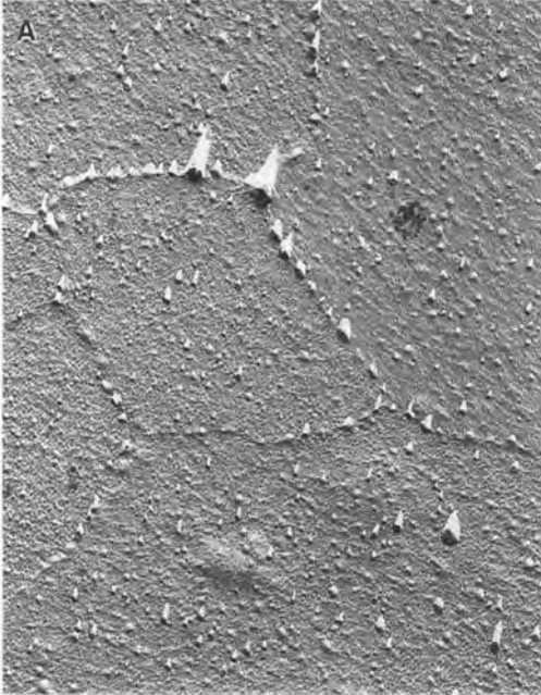
Figure 56. Scanning electron micrograph of a fractured surface of an ex-reactor LWR \text{UO}_2 fuel pellet, recorded close to the fuel centre, showing very high grain boundary porosity and a high density of spherical precipitates of the metallic fission products.
