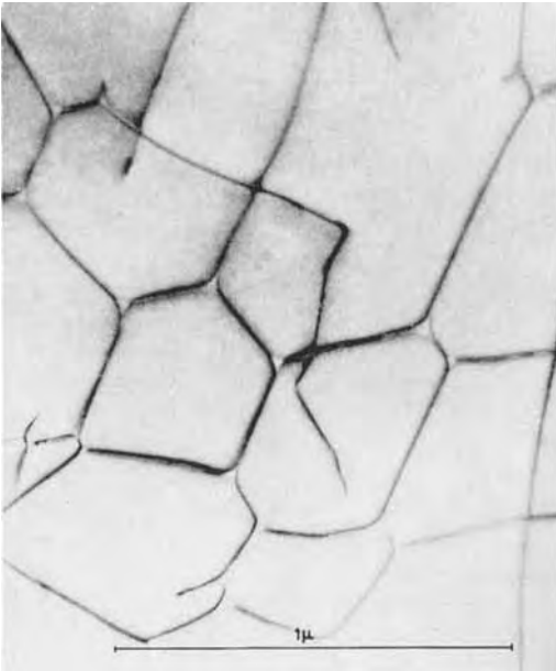
Figure 99. Network of extended dislocations in silicon; all nodes are dissociated. (Courtesy of E. Aerts.)
