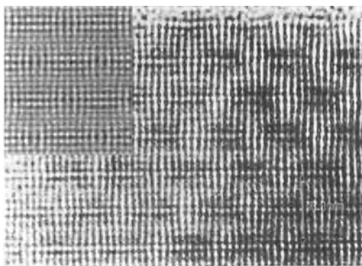
Figure 23. HREM of the n = 1 phase of BSCCO, viewed along the [110] direction. Both the (001) and (110) planes exhibit a wavy character. The computed image, for a model exhibiting an excess oxygen shows good correspondence with the experimental micrograph.
