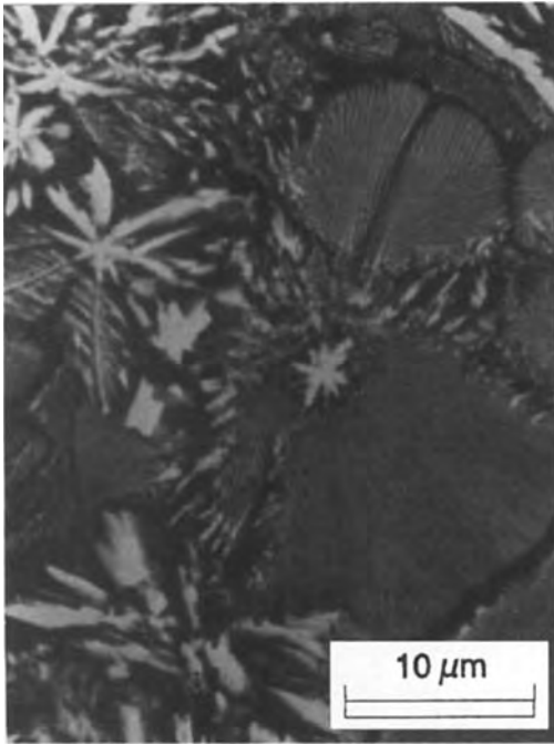
Figure 10. Microstructure of a BMAS glass-ceramic, heat treated at 1070°C for several hours. Quantitative compositional EPMA indicated the presence of fine, interpenetrating, white celsian and black cordierite crystals, in combination with isolated barium osumilite crystals. A small amount of residual glass surrounds the crystalline phases. Back-scattered electron detector image ( \times 2000 ).
