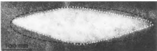
Figure 16. Micrograph of a t\text{-ZrO}_2 precipitate in Mg-PSZ with an oblate ellipsoid, having the same principal axes.
