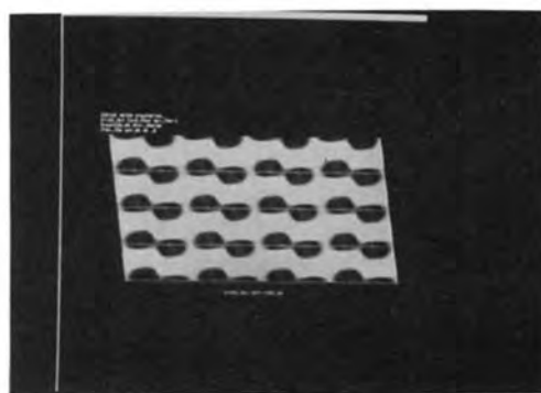
Figure 57. Simulated images obtained from model structures for different defocus ( \Delta f ) and thickness ( t ) values.
