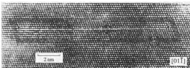
Figure 26. Glide ribbon consisting of Shockley partials separated by an intrinsic stacking fault (Burgers circuits are outlined). Such ribbons are used as probes to measure the stacking fault energy (HREM) (Luyten et al. [97]).
