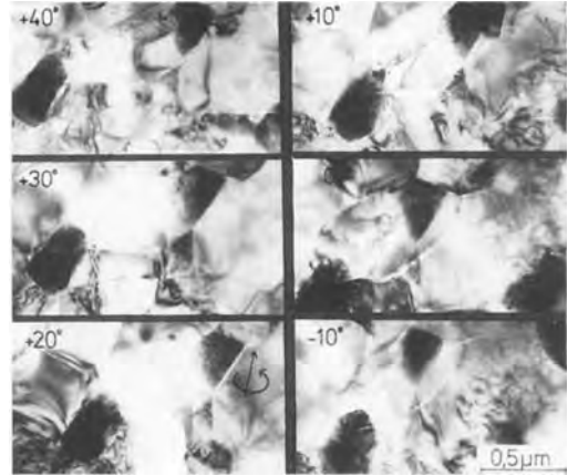
Figure 22. A tilting sequence indicating the technique used to trace microcracks.
