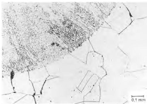
Figure 22. Reheat cracks in the HAZ of a weld in a coarse-grained austenitic stainless steel 1.4550 (field metallographic replica technique).
