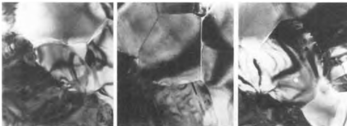
Figure 20. Three examples of microcracks observed at twin terminations in the \text{Al}_2\text{O}_3/\text{ZrO}_2 interface.
