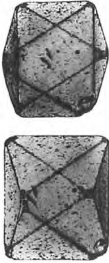
Figure 18. X-ray topographs illustrating the perfection of certain diamonds (Lang [63]).
