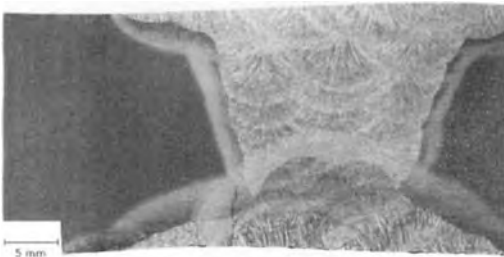
Figure 24. Environmentally assisted (strain-induced) cracking in the repair weld and HAZ of a quenched and tempered ferritic tube weld (material 15NiCu-MoNb 5).
