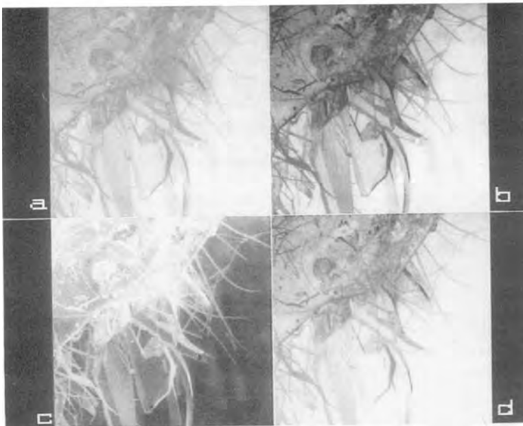
Figure 5. Illustration of global image preprocessing by the histogram-manipulation approach (here, histogram stretching is used as an example). (a) Initial image of whiskers with low contrast. (b) Image resulting from histogram stretching. (c) Contrast inversion of (c). (d) Anamorphosis (logarithmic transfer function) of (a).
