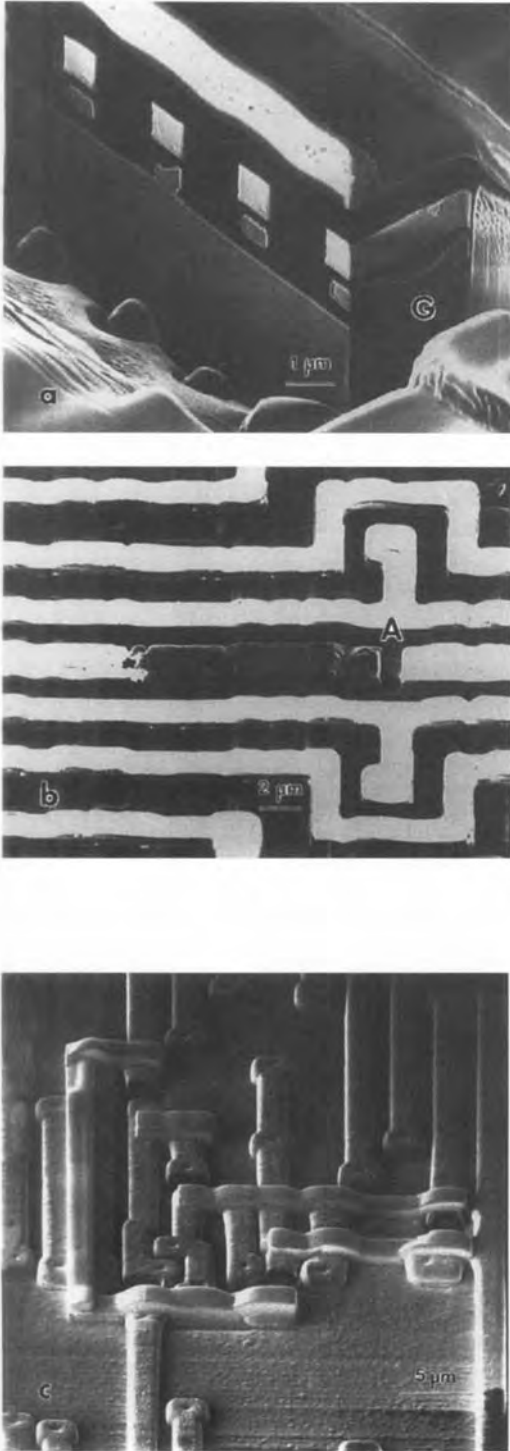
Figure 39. Focused ion beam application in failure analysis. (a) FIB image of precision cross-section etched by FIB. (b) FIB image of aluminum interconnections. The interruption is visible because of local charging. (c) Ion-beam-induced deposition of metal interconnections (horizontal lines).
