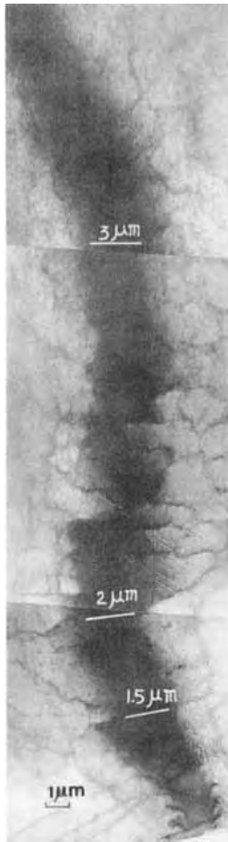
Figure 2. Thickness effect on the formation of cell structures in aluminum [4]. The wedge-shaped specimen was deformed by HVEM to form cell structures, and the micrograph was taken at 0.5 MV. Local thicknesses of the specimen are indicated in the micrograph.
