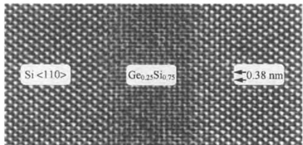
Figure 12. Lattice image of \text{Si}/\text{Si}_{0.75}\text{Ge}_{0.25}/\text{Si} quantum well structure viewed in (110) cross-section. Reproduced by permission of P. Schwander et al. [42].
