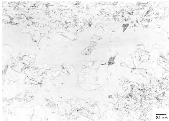
Figure 21. Partially recrystallized microstructure in a forging of stabilized austenitic stainless steel 1.4550.
