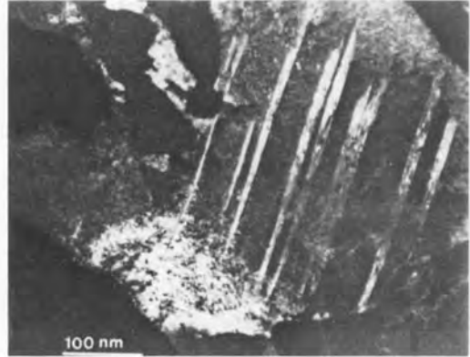
Figure 11. Wear induced \alpha -martensite near the surface.
