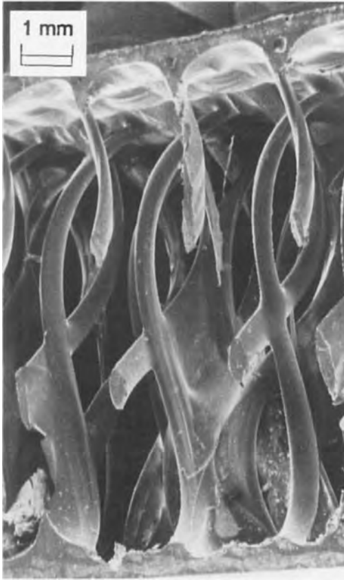
Figure 14. SEM image ( \times 10 ) of the core of a three-dimensional woven sandwich fabric composite. The shape of the connecting pile fibers depends on the production process, and can be quantified using microscopy techniques.
