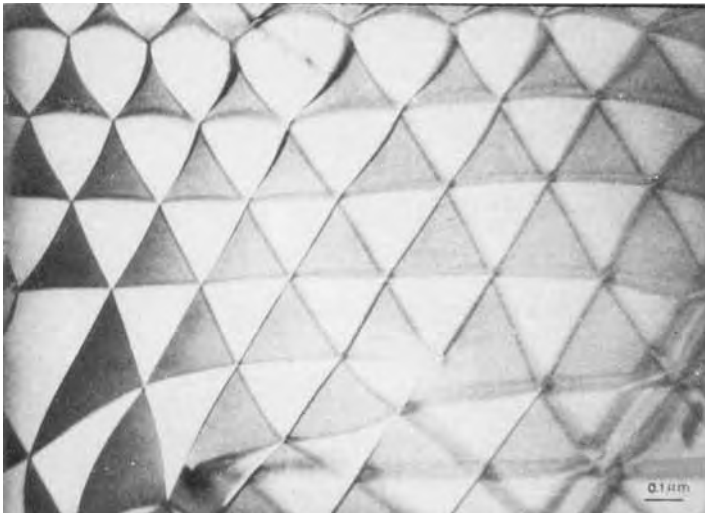
Figure 35. Inversion domains in the \chi phase of Fe-Cr-Mo-Ti revealed by domain contrast [31].
