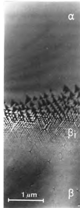
Figure 24. The phase front between the \alpha - and \beta -phases in quartz is observed to consist of a regular array of pyramidal Dauphiné twins forming an incommensurate modulated structure, the period of which reduces as the \beta -phase region is approached. The specimen is close to 573°C; there is a gradient of a few degrees across the area of the photograph.
