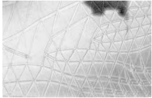
Figure 40. Inversion domains in the \chi phase of Fe-Cr-Mo-Ti, as revealed by interface contrast [34].
