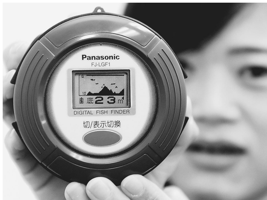
A digital fish finder, the display of which is made with the use of liquid crystal diodes.
