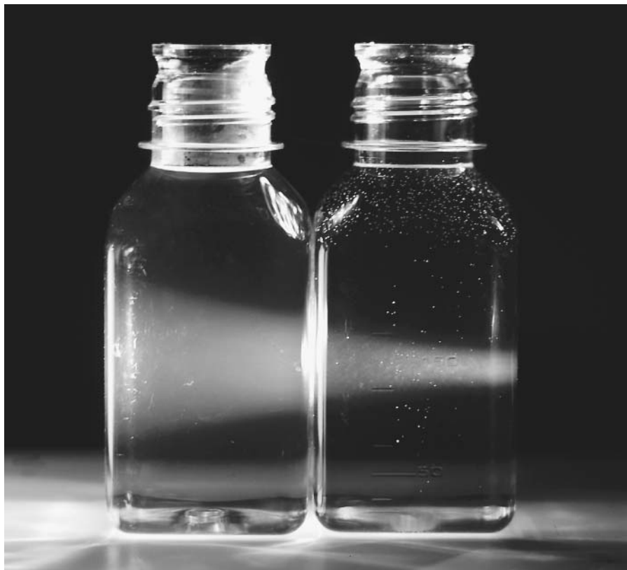
Light passing through a bottle containing sodium hydroxide (NaOH, left), and a bottle containing a colloidal mixture (right).
