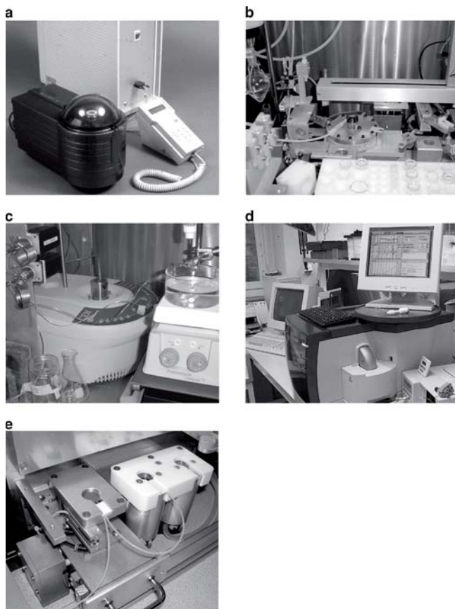
Fig. 1. Commercially supplied single-mode microwave cavities being used in PET. (a) The Microwell 10 (Labwell AB, Uppsala, Sweden) with a footprint of 18 \times 34 \times 30 cm (w \times d \times h). (b) The Model 521 (Resonance Instruments Inc., Skokie, Ill., USA, diameter=15 cm) shown here in a hot cell at NIMH (provided by Shui-Yu Lu). (c) The Discover (CEM, Matthews, N.C., USA; 36 \text{ cm} \times 44 \text{ cm} \times 22 (w \times d \times h)) is shown here integrated in a hot cell at NIMH (provided by Shui-Yu Lu). (d) The SmithCreator (Biotage, Uppsala, Sweden) shown here in a laboratory environment (provided by Hans Ehrsson). (e) The custom-designed 600-W microwave cavity (Scansys Laboratorieteknik, Værløse, Denmark) integrated into a modular PET radiosynthesis system (provided by Peter Larsen)
