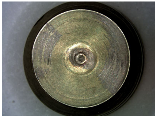
Fig. 3.9 Left: notching of a Ti6Al4V spine rod as the result of contouring prior to placement in the body. Other marks are due to the locking heads of the pedicle screws. Scratching as a result of fitting the rod in the pedicle screws is also evident. Right: wear damage from pedicle screws on a CoCrMoC (ASTM F75 wrought alloy) rod. Burnished mark above the wear is Ti6Al4V from the tulip heads smeared onto the rod
