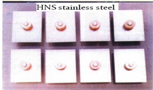
Fig. 6.19 Specimen setup for the field test in the sea
