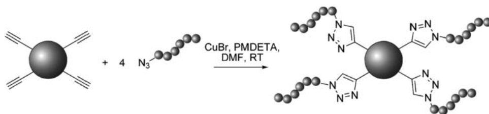
Scheme 6.9 The synthesis of an A_4 star polymer via the CuAAC approach using typical reaction conditions.
