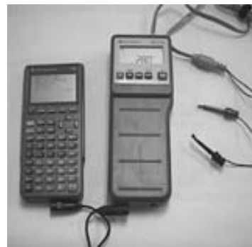
Vernier Voltage Probe Photograph Courtesy of Vernier Software & Technology
