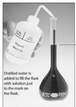
A mark on the neck of a volumetric flask indicates a volume of exactly 250 mL at 25 °C.
