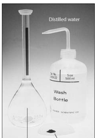
250 mL volumetric flask 0.435g \text{KMnO}_4
