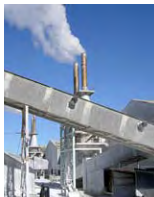
Heated to high temperature in an industrial plant, calcium carbonate, \text{CaCO}_3 , is quickly converted into lime, \text{CaO} , and carbon dioxide.
