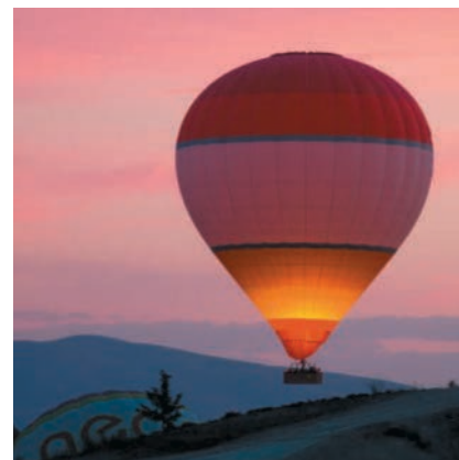
▲ A hot-air balloon floats because the hot air within the balloon is less dense than the surrounding cold air.
