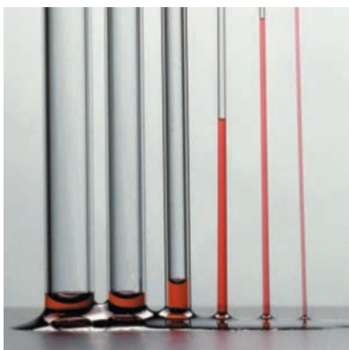
▲ FIGURE 11.18 Capillary Action The attraction of water molecules to the glass surface draws the liquid around the edge of the tube up the walls. The water in the rest of the column is pulled along by the attraction of water molecules to one another. As can be seen in this figure, the narrower the tube, the higher the liquid will rise.
