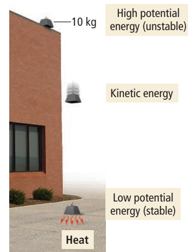
▲ FIGURE E.6 Energy Changes Gravitational potential energy is converted into kinetic energy when the weight is released. The kinetic energy is converted mostly to thermal energy when the weight strikes the ground.
