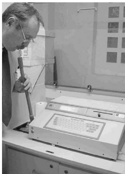
Fig. 23.4 Measuring alcohol molecules by infrared absorption. The instrument is a Lion Intoxilyzer 6000, manufactured by Lion Laboratories, Barry, South Wales.
