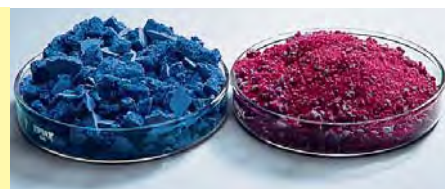
When blue anhydrous \text{CoCl}_2 reacts with water, pink \text{CoCl}_2 \cdot 6\text{H}_2\text{O} is formed.
