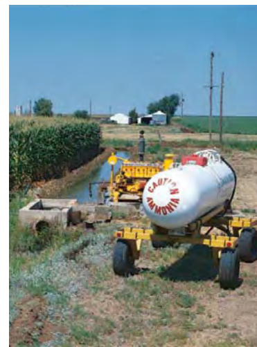
Ammonia being dissolved in irrigation water to provide fertilizer for a field of corn
