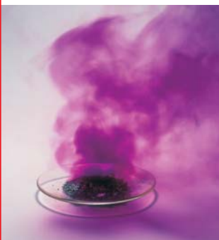
Aluminum (left) and iodine (right) shown at the top, react vigorously to form aluminum iodide. The purple cloud results from excess iodine vaporized by the heat of the reaction.
