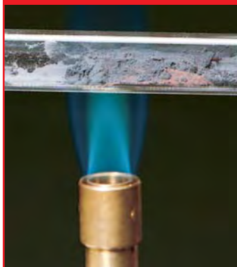
Copper(II) oxide reacting with ammonia in a heated tube
