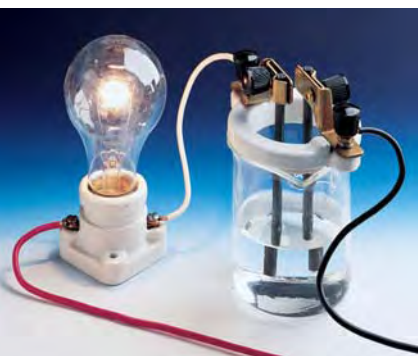
A hydrochloric acid solution readily conducts electric current, as shown by the brightness of the bulb.
