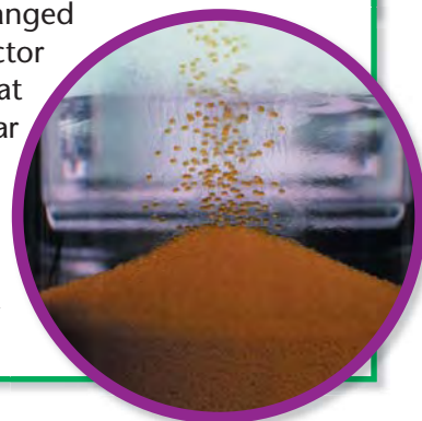
Uranium-238 kernels for use in a reactor
