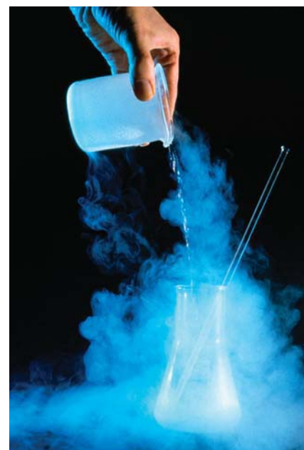
Nitrogen, which forms a liquid at 77 K, is being poured causing moisture in the air to freeze to produce a fog.
