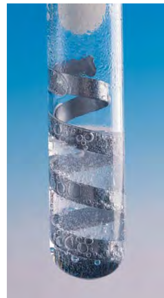
Zinc metal reacts with hydrochloric acid to produce bubbles of hydrogen gas.
