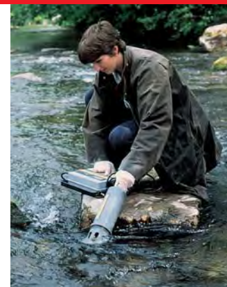
Measuring the pH of the water in a river
