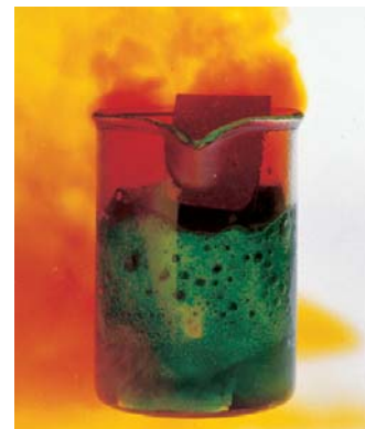
Copper metal reacting with concentrated nitric acid. The solution is colored by the presence of \text{Cu}^{2+} ions. The brown gas is \text{NO}_2 .
