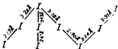
Structure of I_9^- ion in [(CH_3)_4N]^+I_9^-
