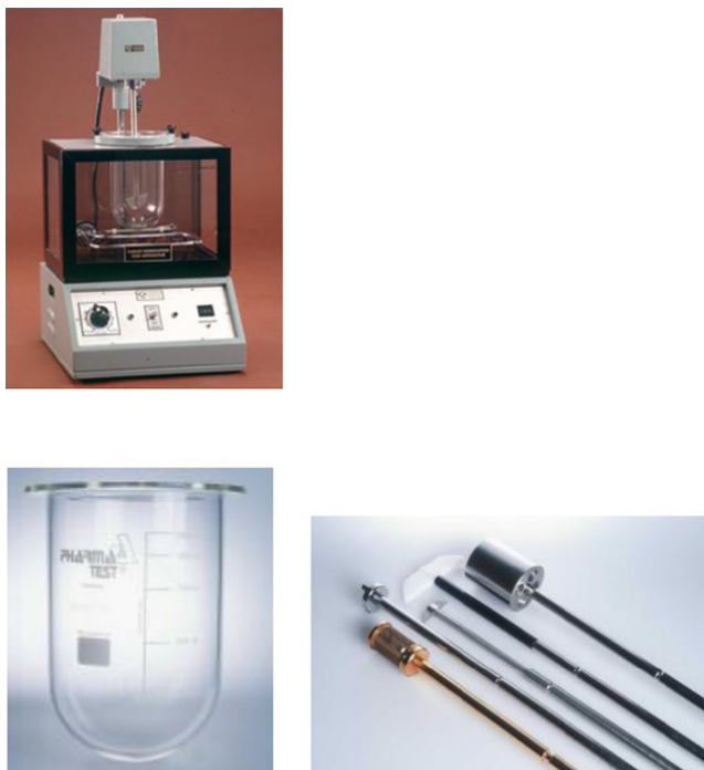
FIGURE 2.9 Typical dissolution apparatuses. http://www.lasany.org/pharma_lab equipments/dissolutiontestapparatus.html , http://www.cecilinstruments.com/autodis-accs.html www.bestlab.com.au/disso_access.htm
