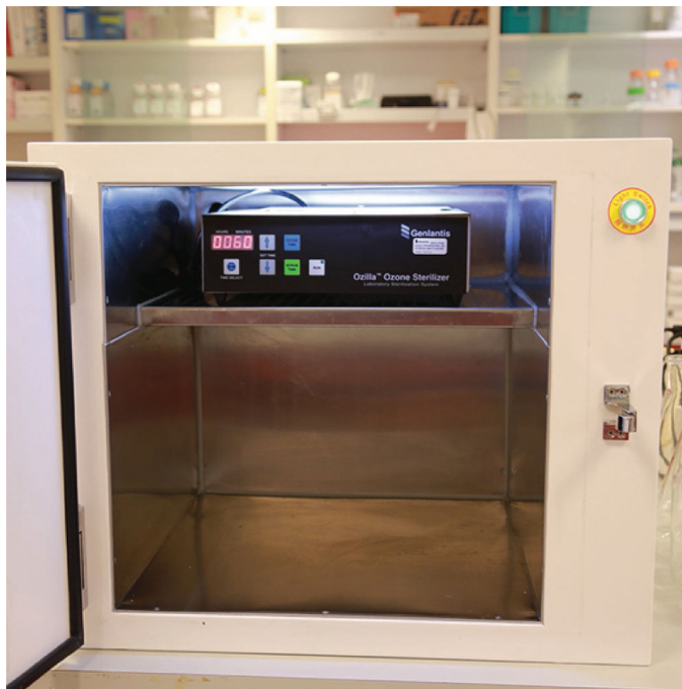
FIGURE 14.23 Ozone sterilization system. Source: Courtesy of Genlantis.
