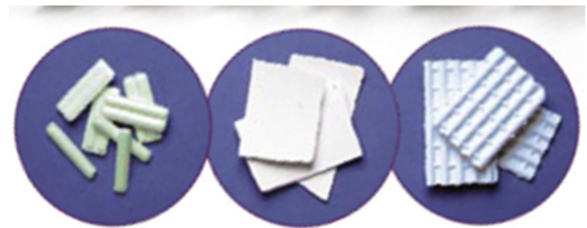
FIGURE 4.6 Examples of product produced from rollers with different surfaces. Courtesy: The Fitzpatrick Co.
