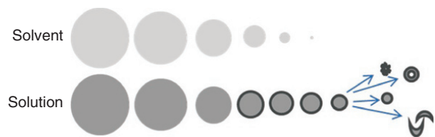
FIGURE 12.12 Drying kinetics of a solvent droplet versus a solution droplet.
