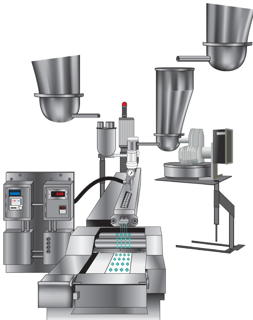
FIGURE 19.4 Direct-to-drug-product extrusion process train schematic, highlighting bulk feeders, precision loss in weight feeders, liquid injection, and calendaring of tablet between two chilled rolls.
