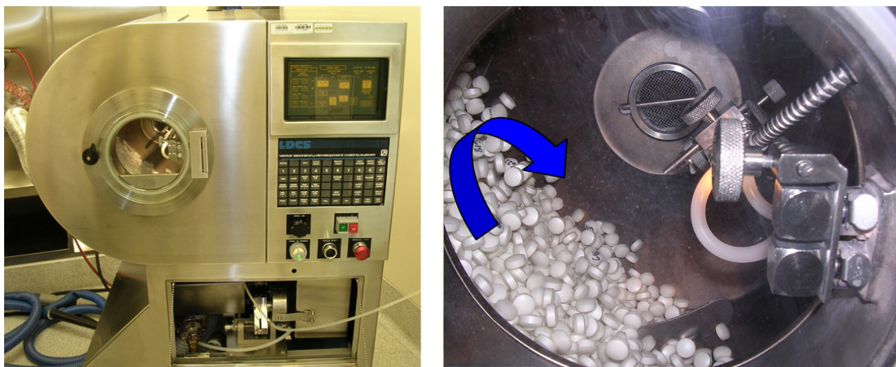
FIGURE 11.2 Left – external view of Vector corp. laboratory development coating system (LDCS 20/30). Right – internal close-up view of cascading tablets during a development coating run. Note: In the image above on the right, a clear coating is added to white tablets. Numbers have been added in order to track individual tablets during the development coating run. The arrow indicates the direction of tablet movement.
