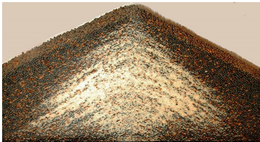
FIGURE 3.4 Example of sifting segregation in a 2-D pile. Note the gray and orange particles are approximately 1200 \mu\text{m} , while the light yellow particles are approximately 350 \mu\text{m} . Source: Courtesy of Jenike & Johanson, Inc.
