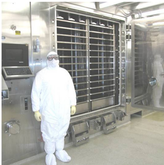
FIGURE 13.4 Image of typical commercial-scale freeze dryer. This freeze dryer has a total shelf surface area of 39 m 2 . It has 24 shelves and 6 trays per shelf. This image is obtained from Pfizer Kalamazoo manufacturing facility.
