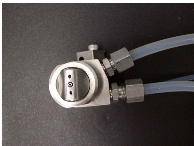
FIGURE 11.6 Front view of a laboratory-scale spray gun for tablet coating (Schlick fluid nozzle and air cap with spray gun body by Vector Inc.).
