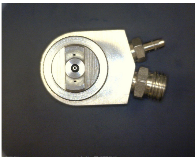
FIGURE 11.8 Front view of a laboratory-scale spray gun for tablet coating (Spraying Systems fluid nozzle and air cap with spray gun body by Vector Inc.).
