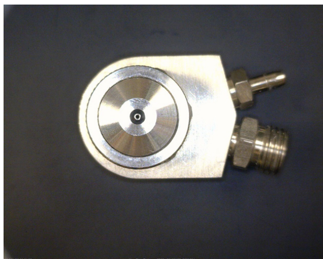
FIGURE 11.10 Side view of a laboratory-scale spray gun for tablet coating (Spraying Systems fluid nozzle and air cap with spray gun body by Vector Inc.).
