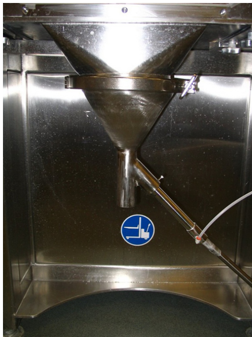
FIGURE 21.15 FBRM with purge tip installed on the Gerteis Macropactor.
