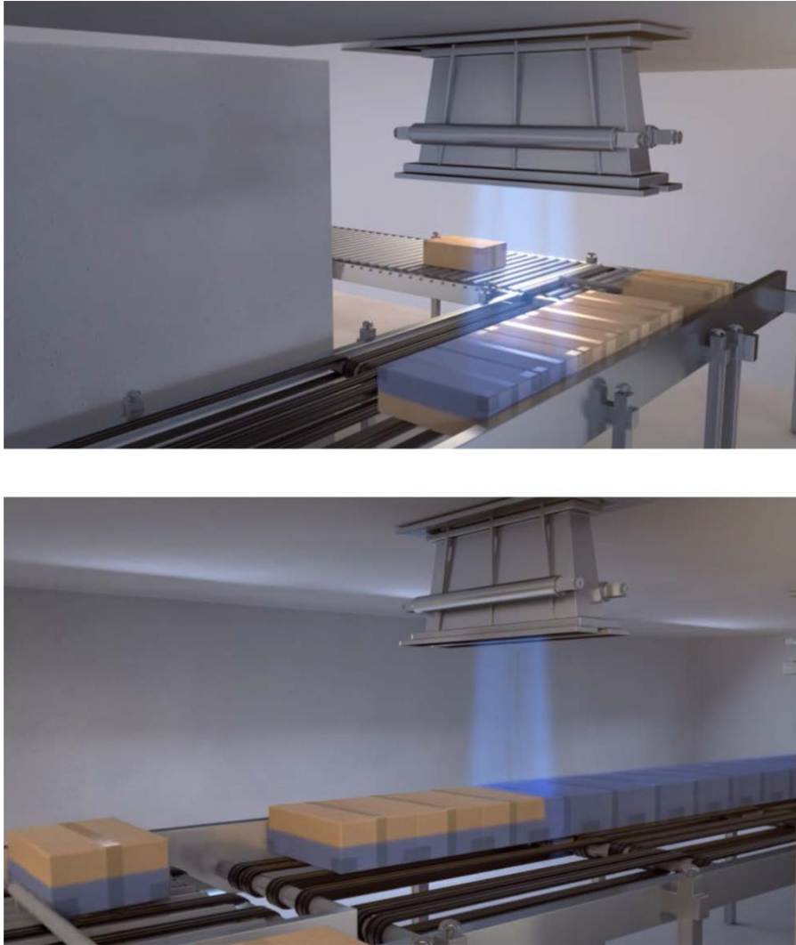
FIGURE 14.15 Sterilization system using E-beam: front irradiation (top panel) and back irradiation (bottom panel) of large packages. Source: Courtesy of Rhodotron, IBA.
