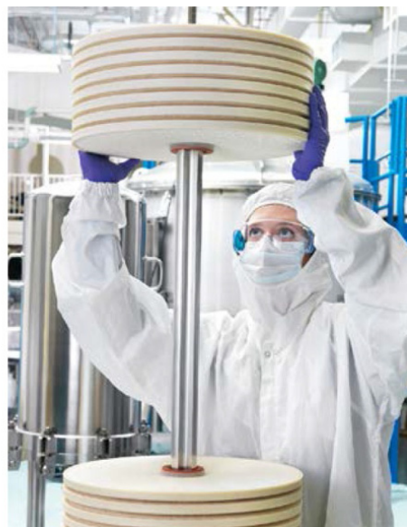
FIGURE 14.28 Lenticular style depth filter cartridges (Millistak+® Depth Filters: left) and their assemblage (right). Source: Both images Courtesy of MilliporeSigma.
