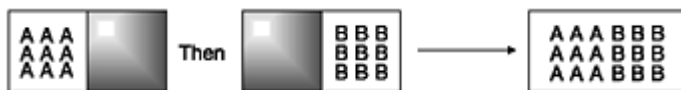
Figure 1.8 Photolithographic synthesis of peptide arrays. In this illustration, one field is covered while the other is reacted with A. Next, the mask is shifted and the uncovered field is reacted with B. Many different patterns can be used so that at the end of an iterative process each location has a different peptide. Thousands of different peptides can be generated in an amazingly small area.
