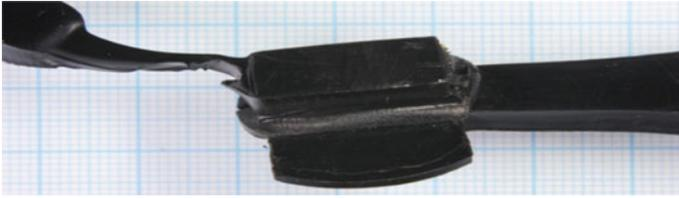
**Fig. 11** Lap-welded joint after mechanical test
