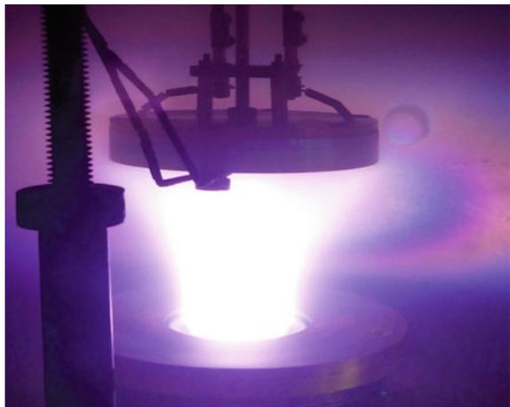
power circuits. Power for the oven is provided by mean of laboratory stabilized switched-mode power supplies BVP 900–1500 W with high currents (10 s A).
