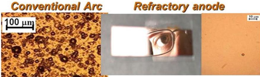
Fig. 15 Comparison of Cu film with conventional and by HRAVA deposition
