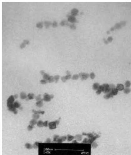
Fig. 10.6 Pd colloids stabilized by microgel. Reprinted from Ref. [19] with permission from Elsevier.
