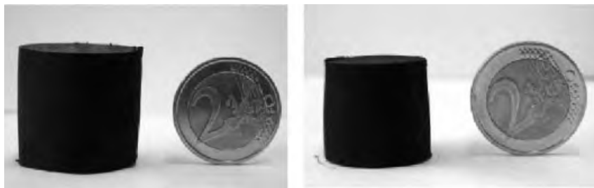
Fig. 7.5 Optical micrographs illustrating the isotropic shrinkage of the cylinder of self-supported multi-walled carbon nanotubes after wetting with water and slow drying in air at room temperature.
