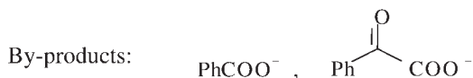
Scheme 13.4 Reaction products detected during the oxidation of phenylethane-1,2-diol (P) with Au/C catalyst. [P]=0.4 M, P/Au=500, P/NaOH=1, T=70 °C.
