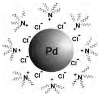
Fig. 2.10 Structural representation of NR 4 X-stabilized metal organosols. Reproduced with permission from Elsevier Science [91].
