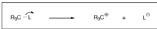
Scheme 5.1 Initial phase of an S_N1 reaction involves dissociation of a leaving group from the starting molecule, generating a carbocation.
