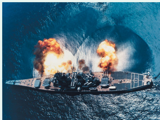
Spherical shock waves generated by the firing of the huge guns of the USS Iowa are clearly visible on the ocean surface.
