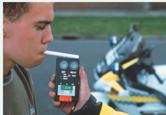
Testing breath for the presence of alcohol.
