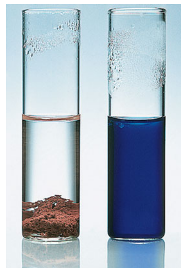
Addition of a molecule containing an aldehyde group to a solution of blue copper(II) sulfate (right) causes the formation of a brick-red precipitate of copper(I) oxide in the Fehling test.
