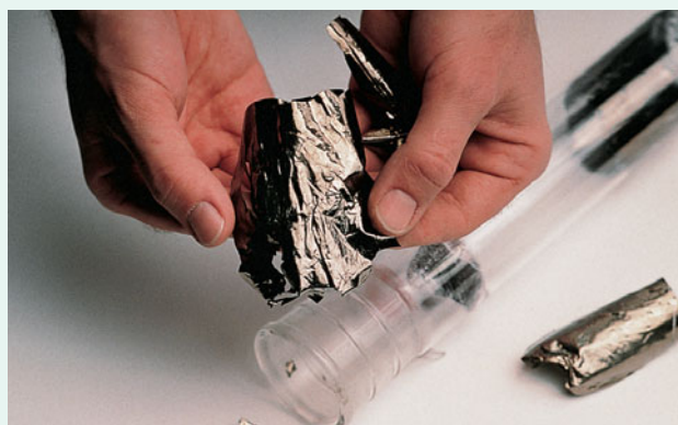
The black, shiny, flexible foil of polyacetylene (polyethyne) made by polymerization of gaseous ethyne on the walls of the reaction vessel shown.
