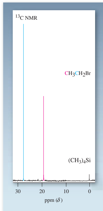
Figure 10-31 This 62.8-MHz ^{13}\text{C} NMR spectrum of bromoethane was recorded with broad-band decoupling at 250 MHz. All lines simplify to singlets, including the absorption for (\text{CH}_3)_4\text{Si} .
