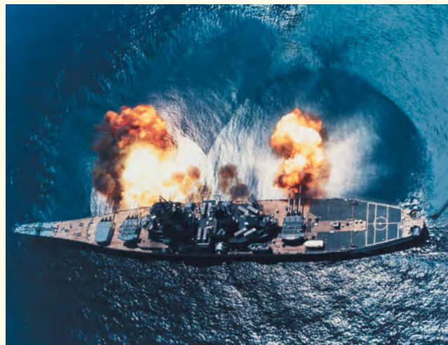
Spherical shock waves generated by the firing of the huge guns of the USS Iowa are clearly visible on the ocean surface.
