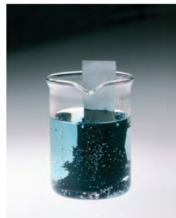
A zinc metal strip reduces a blue \text{Cu}^{2+} salt solution. While the Zn dissolves as \text{Zn}^{2+} , Cu metal forms a black precipitate: \text{Cu}^{2+} + \text{Zn} \rightarrow \text{Cu} + \text{Zn}^{2+} .
