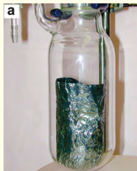
The black, shiny, flexible foil of polyacetylene (polyethyne) made by polymerization of gaseous ethyne.
