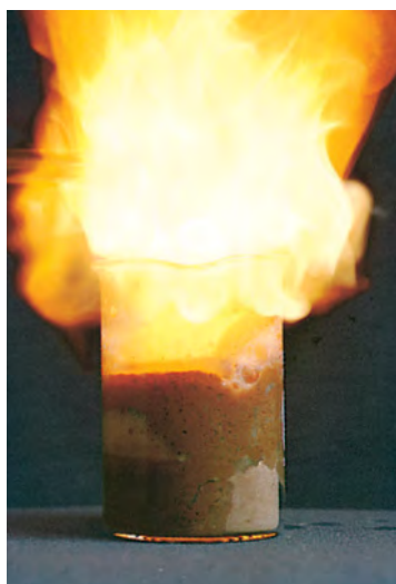
Vivid demonstration of the combustion of ethyne, generated by the addition of water to calcium carbide.
