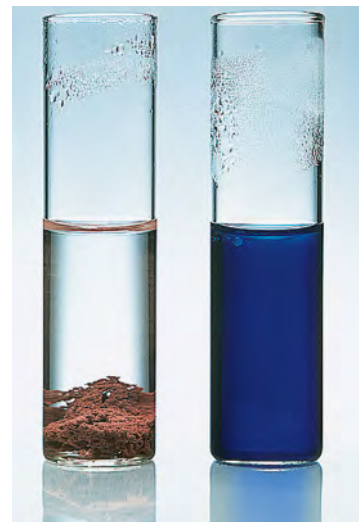
Addition of a molecule containing an aldehyde group to a solution of blue copper(II) sulfate (right) causes the formation of a brick-red precipitate of copper(I) oxide in the Fehling test.
