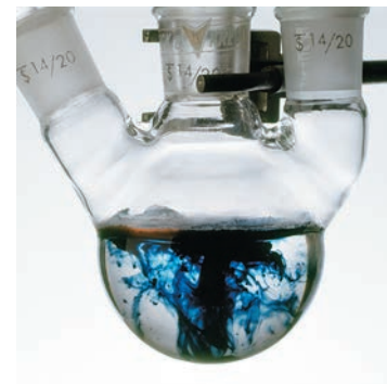
As sodium dissolves in liquid ammonia, it forms a deep blue solution of dissolved \text{Na}^+ and electrons.
