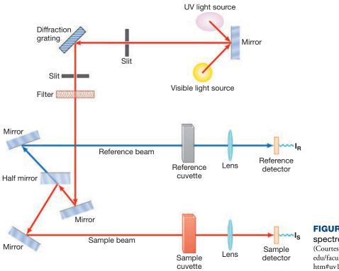
FIGURE 13.8 A diagram of a UV–Vis spectrophotometer. (Courtesy William Reusch, http://www2.chemistry.msu. edu/faculty/reusch/VirtTxtJml/Spectrpy/UV-Vis/uvspec. htm#uv1.© 1999) UV and visible radiation are of higher energy (shorter wavelength) than infrared radiation (used in IR spectroscopy) and radio frequency radiation (used in NMR) but not as energetic as X-radiation (Fig. 13.7).
