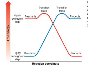
**FIGURE 6.10** The transition state for a highly exergonic step (red curve) lies close to and resembles the reactants. The transition state for an endergonic step (blue curve) lies close to and resembles the products of a reaction. (Reprinted with permission of the McGraw-Hill Companies from Pryor, W., *Free Radicals*, p. 156, copyright 1966.)
