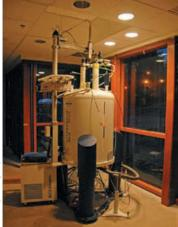
The superconducting magnet of a 500 Mhz FT-NMR spectrometer.
