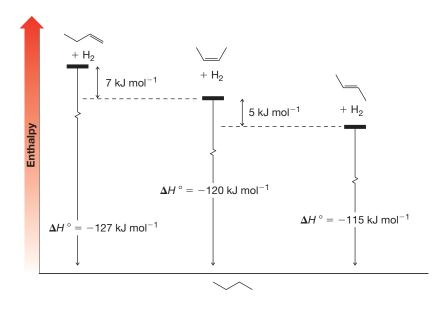
**FIGURE 7.2** An energy diagram for platinum-catalyzed hydrogenation of the three butene isomers. The order of stability based on the differences in their heats of hydrogenation is *trans*-2-butene > *cis*-2-butene > 1-butene.
