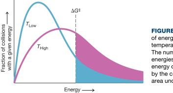
**FIGURE 6.3** The distribution of energies at two different temperatures,  $T_{Low}$  and  $T_{High}$ . The number of collisions with energies greater than the free energy of activation is indicated by the corresponding shaded area under each curve.
