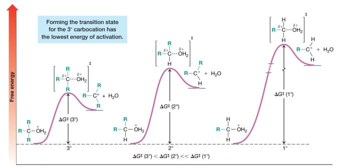
**FIGURE 7.7** Free-energy diagrams for the formation of carbocations from protonated tertiary, secondary, and primary alcohols. The relative free energies of activation are tertiary < secondary << primary.
