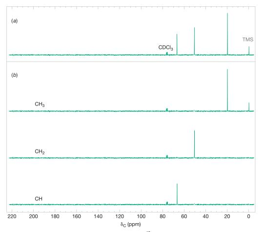
**FIGURE 9.19** (a) The broadband proton-decoupled <sup>13</sup>C NMR spectrum of 1-chloro-2-propanol. (b) These three spectra show the DEPT <sup>13</sup>C NMR data from 1-chloro-2propanol (see Section 9.8D). (This will be the only full display of a DEPT spectrum in the text. Other <sup>13</sup>C NMR figures will show the full broadband proton-decoupled spectrum but with information from the DEPT <sup>13</sup>C NMR spectra indicated near each peak as C, CH, CH<sub>2</sub>, or CH<sub>3</sub>.)
