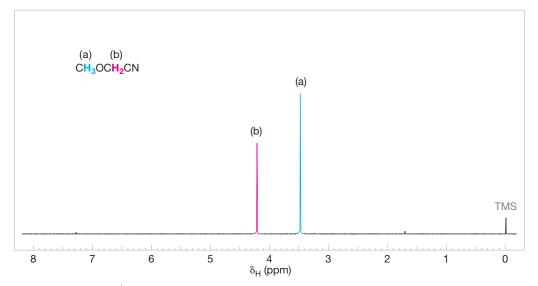
**FIGURE 9.11** The <sup>1</sup>H NMR spectrum of methoxyacetonitrile. The signal of the enantiotopic protons (b) is not split.
