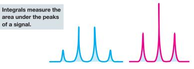
The area under each signal (shown with light blue shading above) is measured (integrated) and taken as a ratio against the area of other signals to compare the relative numbers of hydrogen atoms producing each signal in an NMR spectrum.
