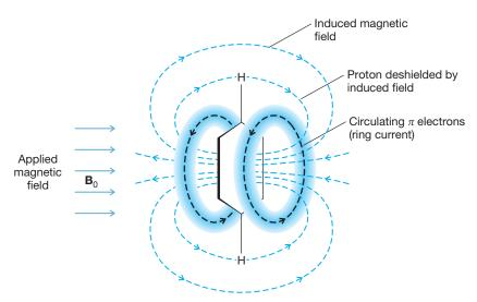
**FIGURE 9.9** The induced magnetic field of the  $\pi$  electrons of benzene deshields the benzene protons. Deshielding occurs because at the location of the protons the induced field is in the same direction as the applied field.
