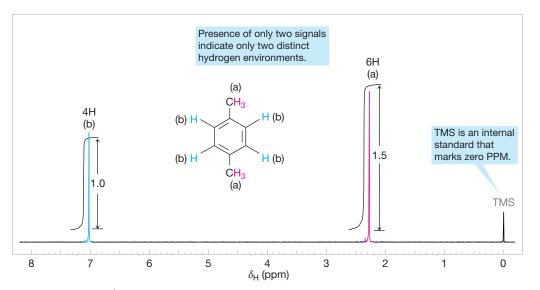
FIGURE 9.3 The <sup>1</sup>H NMR spectrum of 1,4-dimethylbenzene.
