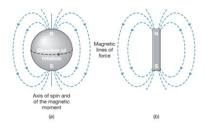
**FIGURE B.1** (*a*) The magnetic field associated with a spinning proton. (*b*) The spinning proton resembles a tiny bar magnet.
