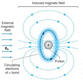
**FIGURE 9.8** Circulations of the electrons of a C—H bond under the influence of an external magnetic field. The electron circulations generate a small magnetic field (an induced field) that shields the proton from the external field.
