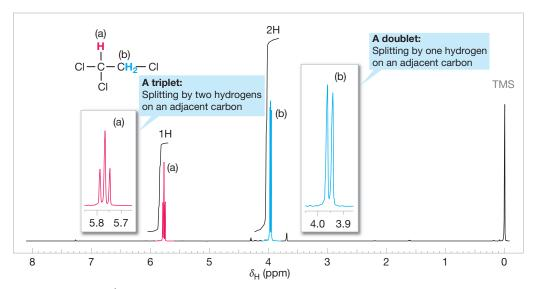
**FIGURE 9.4** The <sup>1</sup>H NMR spectrum of 1,1,2-trichloroethane. Zoomed-in expansions of the signals are shown in the offset plots.
