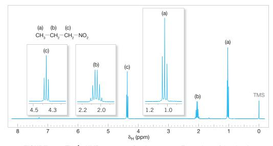
**FIGURE 9.14** The <sup>1</sup>H NMR spectrum of 1-nitropropane. Expansions of the signals are shown in the offset plots.
