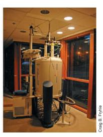
The superconducting magnet of an FTNMR spectrometer.
