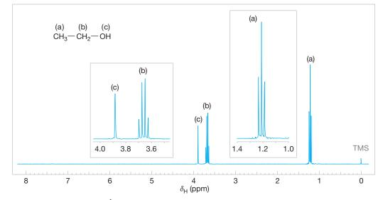
**FIGURE 9.17** The <sup>1</sup>H NMR spectrum of ordinary ethanol. There is no signal splitting by the hydroxyl proton due to rapid chemical exchange. Expansions of the signals are shown in the offset plots.
