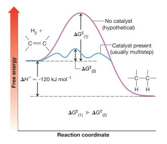
**FIGURE 7.9** Free-energy diagram for the hydrogenation of an alkene in the presence of a catalyst and the hypothetical reaction in the absence of a catalyst. The free energy of activation for the uncatalyzed reaction ( $\Delta G^{\dagger}_{(1)}$ ) is very much larger than the largest free energy of activation for the catalyzed reaction ( $\Delta G^{\dagger}_{(2)}$ ). The uncatalyzed hydrogenation reaction does not occur.
