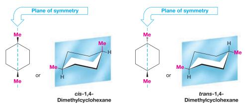
**FIGURE 5.16** The cis and trans forms of 1,4-dimethylcyclohexane are diastereomers of each other. Both compounds are achiral, as the internal plane of symmetry (blue) shows for each.
