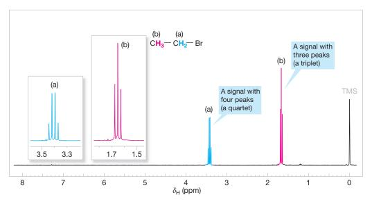
**FIGURE 9.1** The <sup>1</sup>H NMR spectrum of bromoethane (ethyl bromide). Zoomed-in expansions of the signals are shown in the offset plots.
