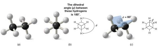
**FIGURE 4.5** (*a*) The staggered conformation of ethane. (*b*) The Newman projection formula for the staggered conformation. (*c*) The dihedral angle between these hydrogen atoms is 60°.
