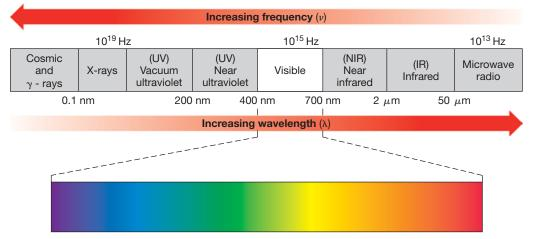
FIGURE 13.7 The electromagnetic spectrum.
