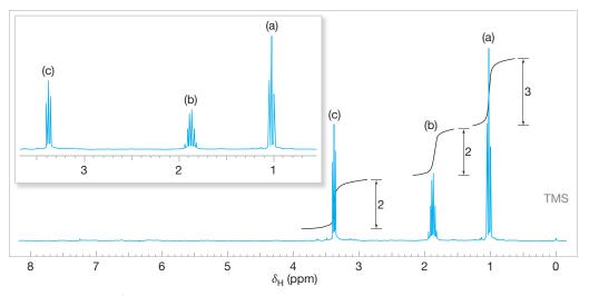
**FIGURE 9.5** The <sup>1</sup>H NMR spectrum of a compound with the formula  $C_3H_7Br$ . Expansions of the signals are shown in the offset plots. (Spectra adapted from Sigma-Aldrich Co. © Sigma-Aldrich Co.)
