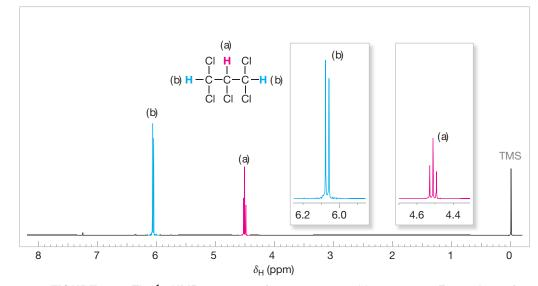
**FIGURE 9.12** The <sup>1</sup>H NMR spectrum of 1,1,2,3,3-pentachloropropane. Expansions of the signals are shown in the offset plots.
