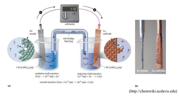
When the cell is completed with a salt bridge, an electrical current begins to flow - what we have is a simple battery (figure a above). Over time, the copper electrode gets heavier as metallic copper is deposited on the copper cathode, while the zinc anode slowly dissolves into solution (figure b above). The redox reaction occurring here is:
