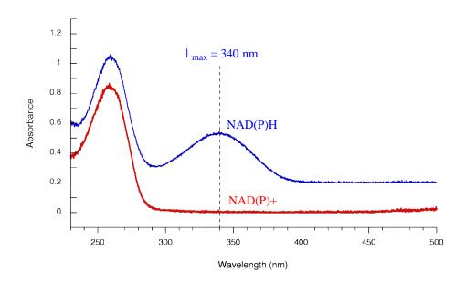
Therefore, the course of a hydrogenation reaction, in which NAD(P)H is converted to NAD(P)<sup>+</sup>, can be observed in real time if it is run in a quartz cuvette in a UV spectrometer. By observing the decrease in absorbance at 340 nm, the researcher can calculate how much NAD(P)H has been oxidized to NAD(P)<sup>+</sup> at any given time point, and this number is the molar equivalent of the amount of organic substrate that has been reduced:
