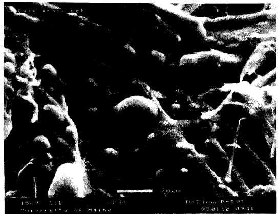
Figure 7.3. High-magnification image of wet-base stock showing the presence of 1–20 \mu\text{m} partially wetting water drops at the fibre surfaces. (From ref. (7) with permission)
