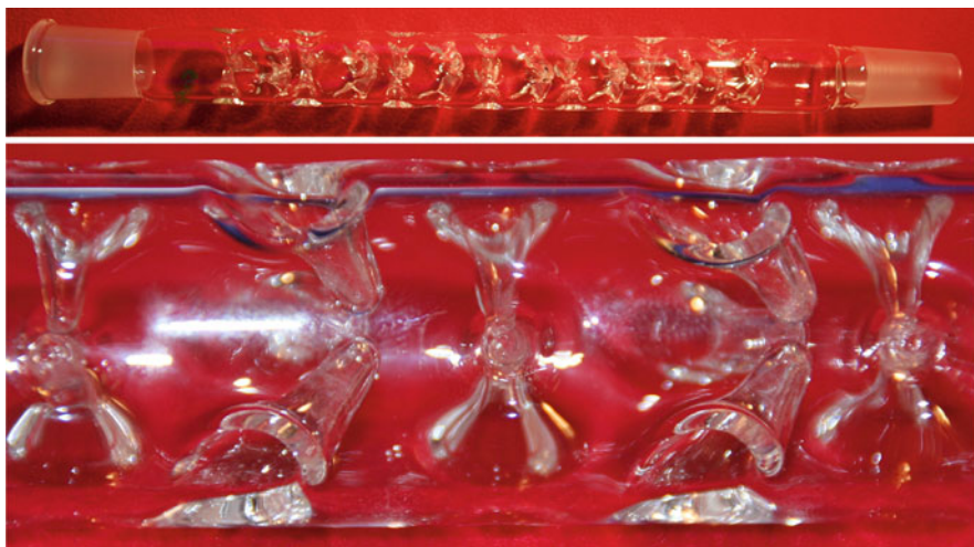
Fig. 3.21 Photograph of a Vigreux fractionation column (top) and close-up of a spike section (bottom)
