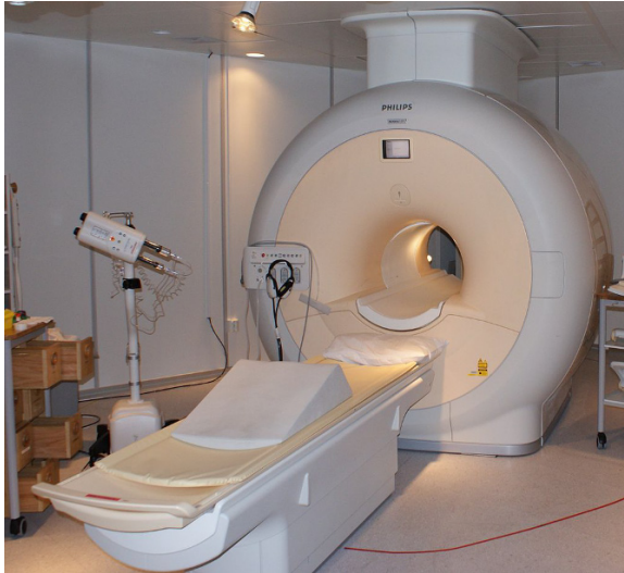
A medical magnetic resonance scanner. The toroidal structure is a superconducting solenoid that produces the dc field. Source: Wikipedia .
