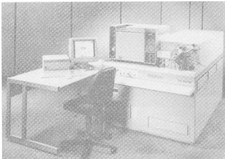
Totally computer controlled mass spectrometer. The inlet system is on the right, with a gas chromatograph in the middle (for GC-MS)
